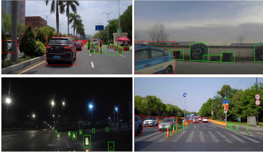
Fig. 3. Representative visual examples from the proposed solution. Noted that the novel objects are drawn in green, while the common objects are drawn in other colors.
