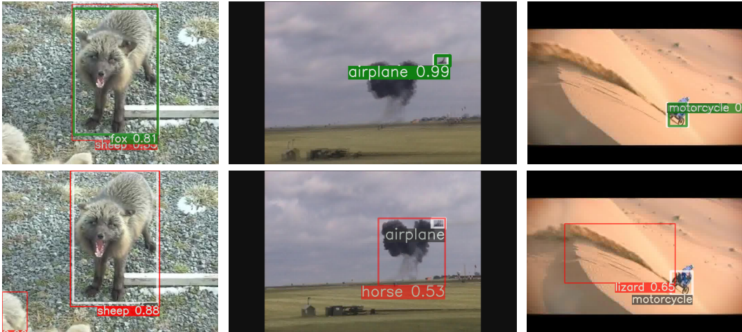
Figure 4: Naturally perturbed examples for detection. Red boxes indicate false positives; green boxes indicate true positives; white boxes are ground truth. Classification errors are common failures, such as the fox on the left, which is classified correctly in the anchor frame, and misclassified as a sheep in a nearby frame. However, detection models also have localization errors, where the object of interest is not correctly localized in addition to being misclassified, such as the airplane (middle) and the motorcycle (right). All visualizations show predictions with confidence greater than 0.5.
