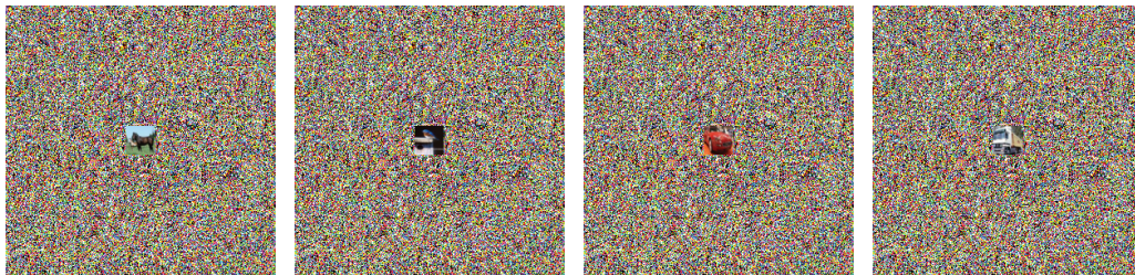
Figure Supp. 1: Examples of adversarial images for CIFAR-10 classification. An adversarial program repurposing an Inception V3 model to classify CIFAR-10 images, applied to four CIFAR-10 images.
