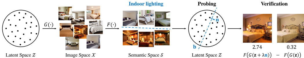
Figure 2: Method for identifying the emergent variation factors in generative representation. By deploying a broad set of off-the-shelf image classifiers as scoring functions, F(\cdot) , we are able to assign a synthesized image with semantic scores corresponding to each candidate variation factor. For a particular concept, we learn a decision boundary in the latent space by considering it as a binary classification task. Then we move the sampled latent code towards the boundary to see how the semantic varies in the synthesis, and use a re-scoring technique to quantitatively verify the emergence of the target concept.
