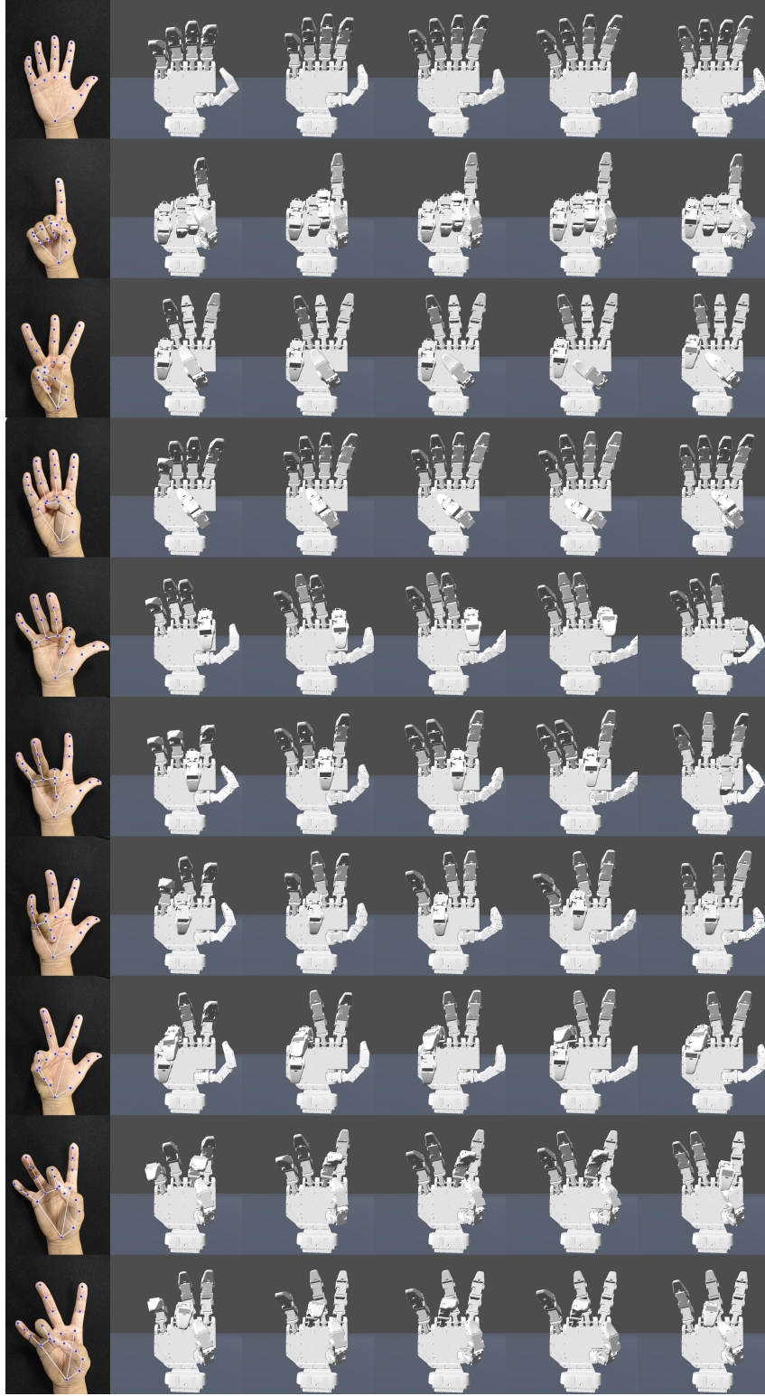
Figure 23: Qualitative Comparison of Retargeting Results on RAPID Hand. From left to right: (1) original human hand gestures, (2–5) results of baseline method [44] using global scaling factors \alpha = 1.25, 1.50, 1.75, 2.00 , and (6) results from our proposed method.
