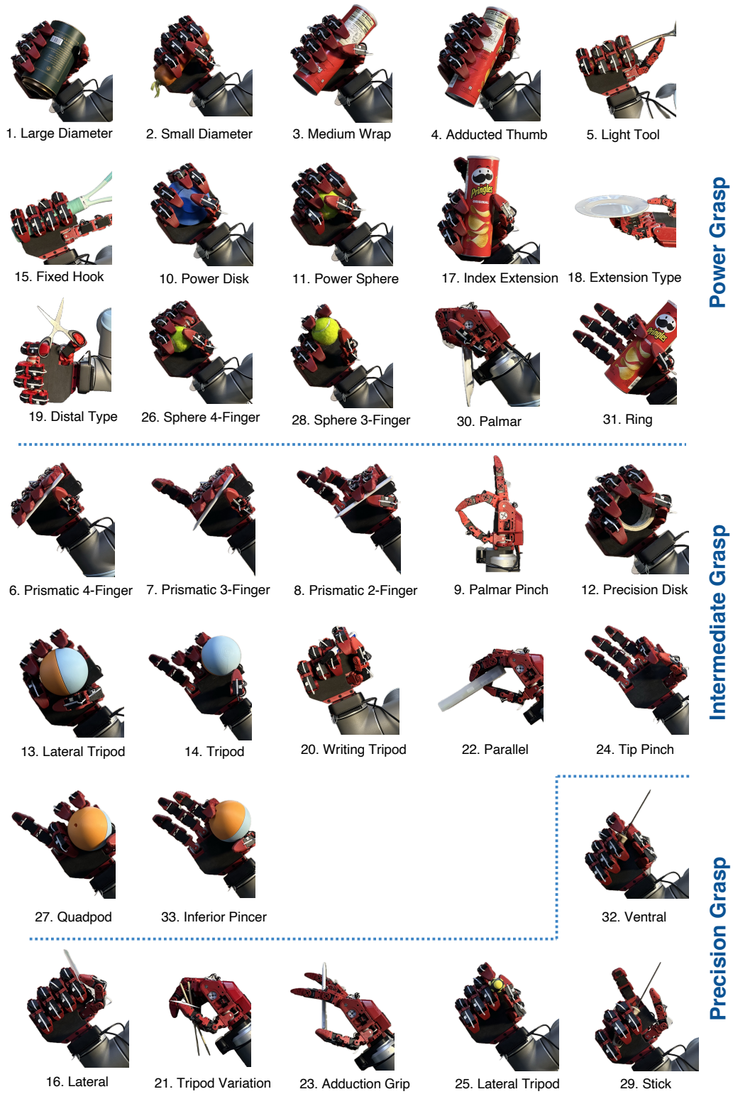
Figure 22: Grasp Taxonomy of the RAPID Hand. Grasp poses and their indices correspond to the Feix taxonomy [51].
