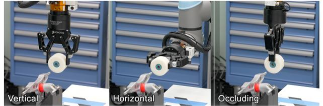
Figure 6. Side-by-side comparison of ID (Vertical) and OOD (Horizontal, Occluding) grasps used in experiments.
