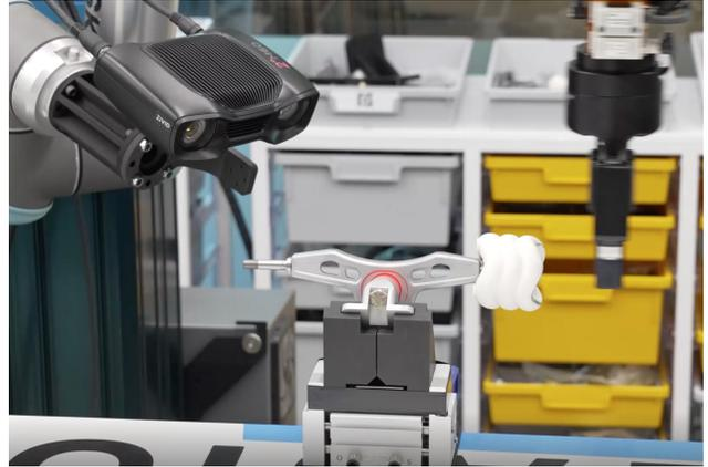
Figure 1. The gripper in Vertical configuration, approaches the Shark wheel at the start of a wheel-on-axle insertion experiment.
