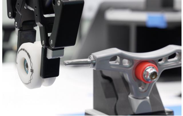
Figure 3. Close-up of fine-tuning dataset generation, showing Small wheel being manipulated by gripper near axle.
