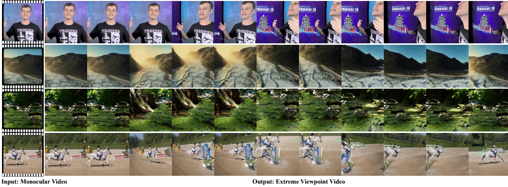
Figure 1: Our EX-NVS framework takes a monocular video as input and generates high-quality videos under extreme viewpoints. By leveraging the proposed Depth Watertight Mesh representation, it effectively handles occlusions in boundaries and ensures geometric consistency, enabling visually coherent and realistic results.
