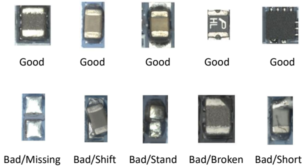
Figure 2: Examples of the input images. 'Good' refers to good soldering. 'Bad' refers to defective soldering. 'Missing,' 'Shift,' 'Stand,' 'Broken,' and 'Short' refers to the defective soldering types.
