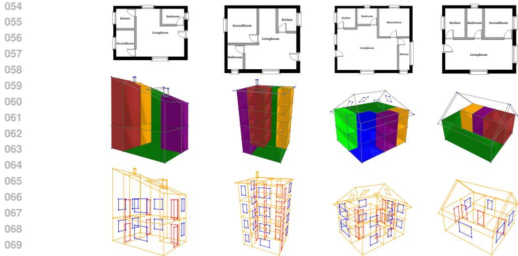
Figure 1: SYNBUILD-3D consists of 103,233 3D building wireframes, floor plan images, and floor plan segmentation masks. Based on the information in each floor plan image (top row), we semantically enrich the corresponding 3D wireframe with information on its room types (middle row) and the position of its doors and windows (bottom row).
