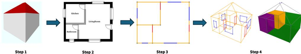
Figure 2: SYNBUILD-3D pipeline. In the first step, a procedural generation engine creates a randomized building exterior. We then use that building’s footprint to produce a building-specific floor plan image (Step 2). Afterward, the floor plan information is vectorized (Step 3) and extruded within the building hull (Step 4).
