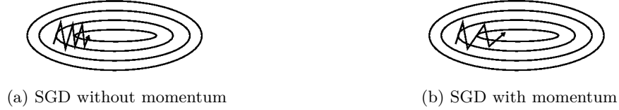
Figure 2: Figures for SGD with and without momentum. This Figure is taken from Ruder (2016) (Figure 2).
