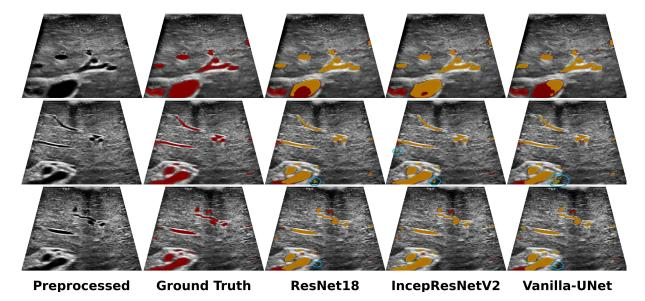
Figure 2. Vessel segmentation results using three models. Red: ground truth, Yellow: model predictions, Blue circles: over-predicted regions.
