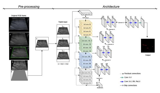
**Figure 1.** Overview of the proposed vessel segmentation pipeline. The raw RGB laparoscopic ultrasound frames undergo five preprocessing steps, are arranged into temporal triplets, encoded with a ResNet18 backbone, and decoded with a U-Net decoder to generate the final binary mask of the vessels.
