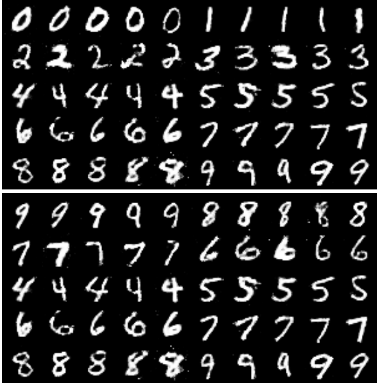
Fig. 2: Redacting labels 0, 1, 2, 3 in cGAN on MNIST. Upper: samples generated from the pre-trained model. Down: samples generated from the redacted model. Redacted conditionals (first two rows) are edited as expected, and other conditionals (last three rows) remain unchanged.
