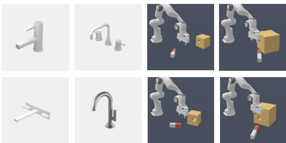
Figure 4. Sampled geometric variations for turn faucet and peg insertion. The sizes of peg / box and the relative locations of the hole vary across different environment seeds.
