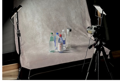
Figure 2: Data collection setup consists of a Canon EOS Rebel T7 camera on the tripod, a table covered with non-reflective cloth backdrop, and LED lights on either side.
