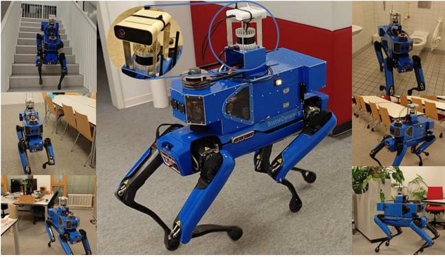
Fig. S.6. Boston Dynamics *Spot* robot traversing a two-story office building with multiple types of rooms. The quadruped is equipped with an Azure Kinect RGB-D camera and a 3D LiDAR. We obtain accurate pose estimates from LiDAR-based odometry estimation.
