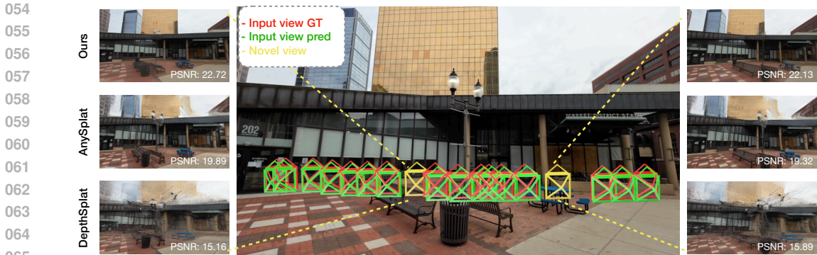
Figure 1: LVSPM can jointly achieve high-quality novel view synthesis and accurate camera pose estimation from uncalibrated long-sequence (128) multi-view images. A subset of the 128 input views with corresponding prediction and ground-truth poses is shown in the middle, while novel view synthesis comparisons are presented on the side. Our estimated poses closely align with ground truth, while our pose-free synthesis results surpass recent baselines, including the pose-free AnySplat (Jiang et al., 2025b) and even the pose-required DepthSplat (Xu et al., 2025b).
