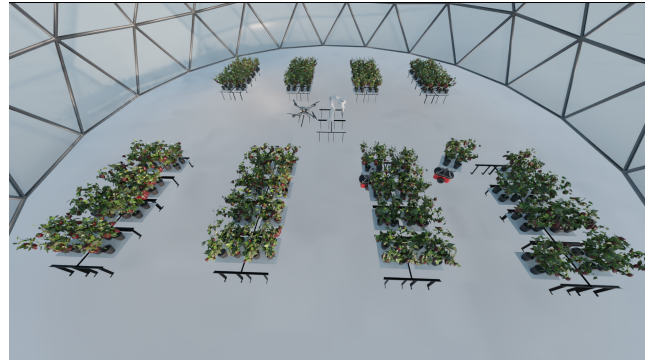
Figure 4: The layout of the proposed greenhouse structure consisting of eight tables, each with four pepper plant containers. The stationary manipulator workstation is located in the center of the structure.
