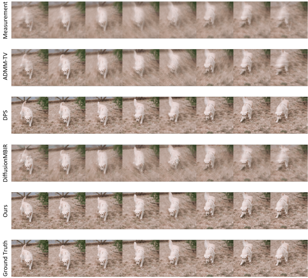
Figure 14: Detailed qualitative comparison in spatio-temporal degradation, including the spatial deblurring ( \sigma=2.0 ) task on the DAVIS dataset, shown with a 2-frame skip.
