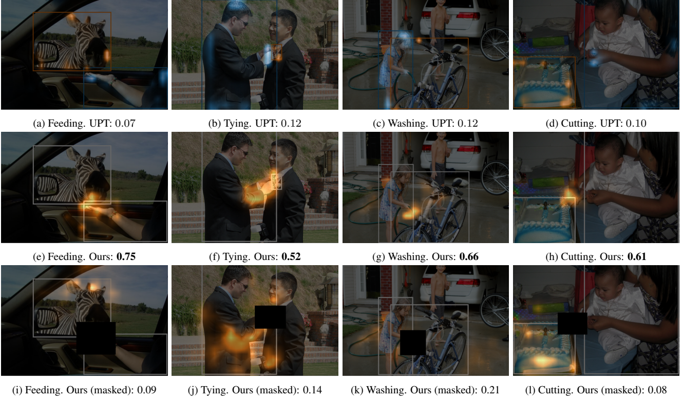
Figure 3. Existing two-stage HOI detectors (e.g., UPT [?]) lack relevant visual context, including (a, b) fine-grained information about the subject or object, such as human pose, and (c, d) other relevant contextual information in the scene, such as another object involved in the interaction. The predicted score for each example is listed in the caption. UPT (first row) uses frozen object features which often pool information from the box boundary since this aids localisation. Consequently, such features do not cover other aspects of the object and are not discriminative enough to recognise complex human–object interactions. Our method (second row) solves such failure cases with spatially guided cross-attention, pinpointing the image regions corresponding to the relevant body parts or the additional object besides the human–object pair. To demonstrate that these regions are indeed highly relevant to the prediction score, we mask out those image regions with the highest attention weights (third row), and observe a significant drop in prediction scores.
