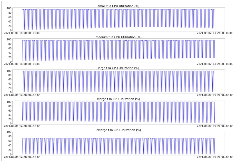
Figure 3: CPU utilization (%) responses on five different EC2 instances (Table 2) from 2PM-UTC 9/1/2021-2PM-UTC 9/2/2021 at 1 minute granularity. This training data was generated internally [4]. The median CPU utilization values (%) are noted to be equal to {95%, 95.5%, 99.5%, 100%, 72.5%}
