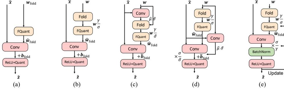
**Figure 3:** Comparison of different Batch Normalization folding technologies. (a) Removing BN layers and directly update  $w_{\text{fold}}$ . (b) BN folding without any statistics update. (c) BN folding with two convolutions. (d) folding with running statistics and also requires two convolutions. (e) folding running statistics with an explicitly BN layer in training. Graph (bcde) can be transformed to (a) during inference. FQuant=FakeQuantize.
