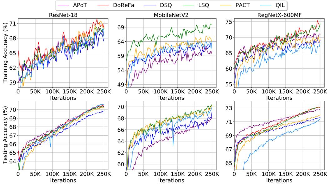
**Figure 7:** Visualization of training and testing accuracy for 6 different algorithms with academic setting on ResNet-18, MobileNetV2 and RegNetX-600MF. Note that DoReFa failed to converge in MobileNetV2 training.
