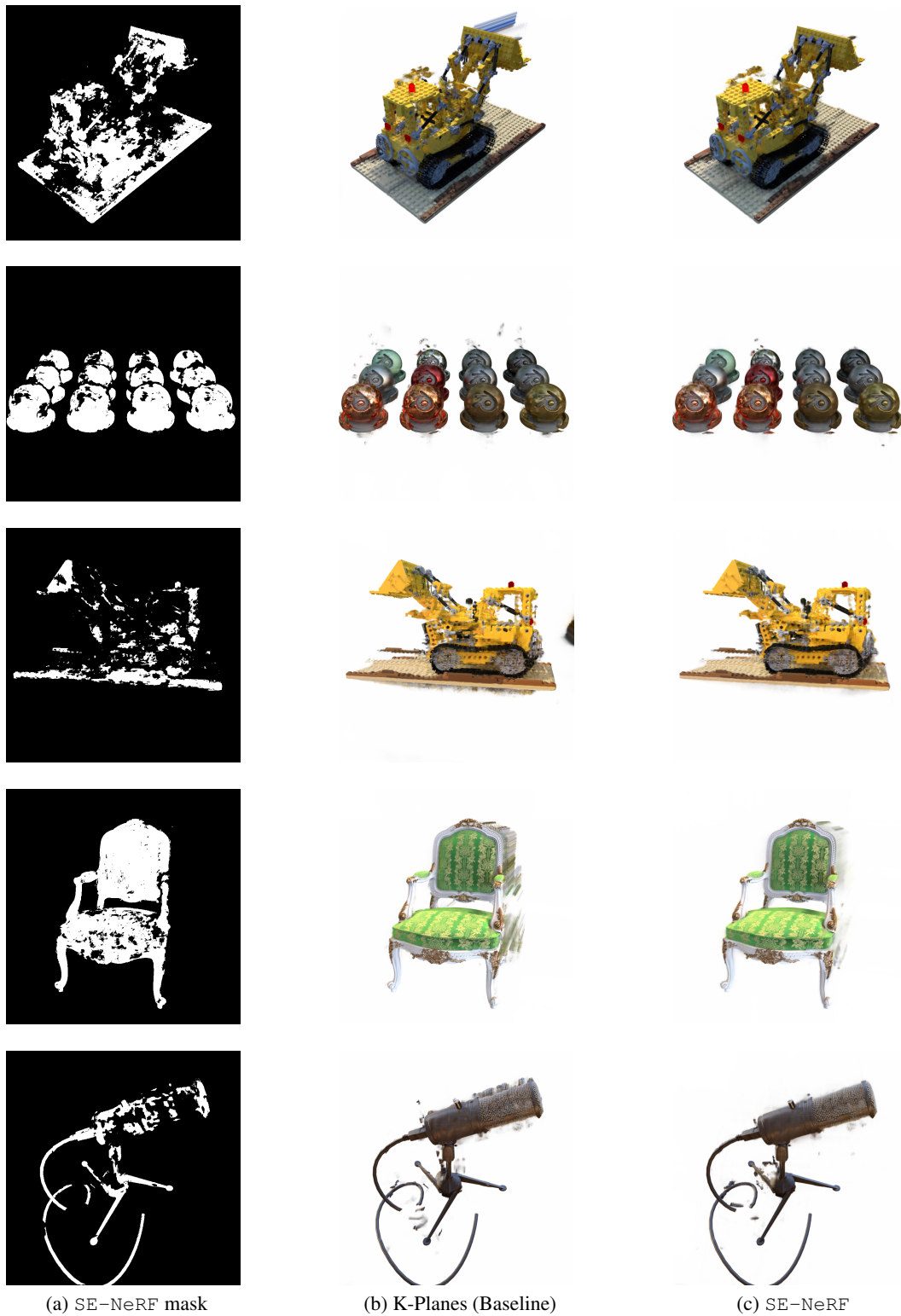
Figure 17: Qualitative improvement from baseline in 3-view setting (NeRF Synthetic Extreme). (a) shows the mask generated by training our model in the 3-view setting using our reliability estimation method. As shown in (c), which presents the results of applying the mask from (a) to (b) in the subsequent iterations of training, we are able to remove the artifacts present in (b) and achieve improved performance.
