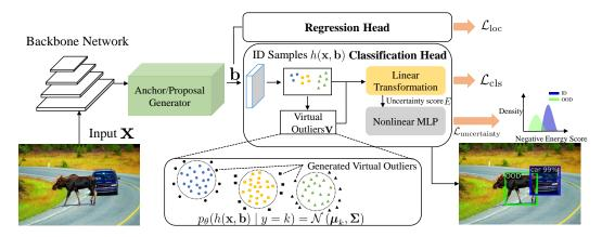
Figure 2: The framework of VOS. We model the feature representation of ID objects as class-conditional Gaussians, and sample virtual outliers  $\mathbf{v}$  from the low-likelihood region. The virtual outliers, along with the ID objects, are used to produce the uncertainty loss for regularization. The uncertainty estimation branch  $(\mathcal{L}_{uncertainty})$  is jointly trained with the object detection loss  $(\mathcal{L}_{loc}, \mathcal{L}_{cls})$ .
