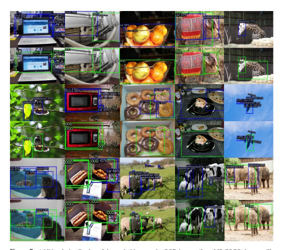
Figure 7: Additional visualization of detected objects on the OOD images (from MS-COCO) by a vanilla Faster-RCNN (*top*) and VOS (*bottom*). The in-distribution is BDD-100k dataset. **Blue**: Objects detected and classified as one of the ID classes. **Green**: OOD objects detected by VOS, which reduce false positives among detected objects.
