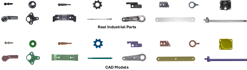
Figure 8: The collected industrial parts and their corresponding CAD models of XYZ-IBD dataset.
