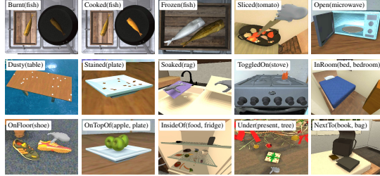
Figure 2: Unary and Binary Predicates in BDDL: We represent object states and relationships to other objects based on their kinematics, temperature, wetness level and other physical and functional properties, enabling a diverse and complex set of realistic activities
