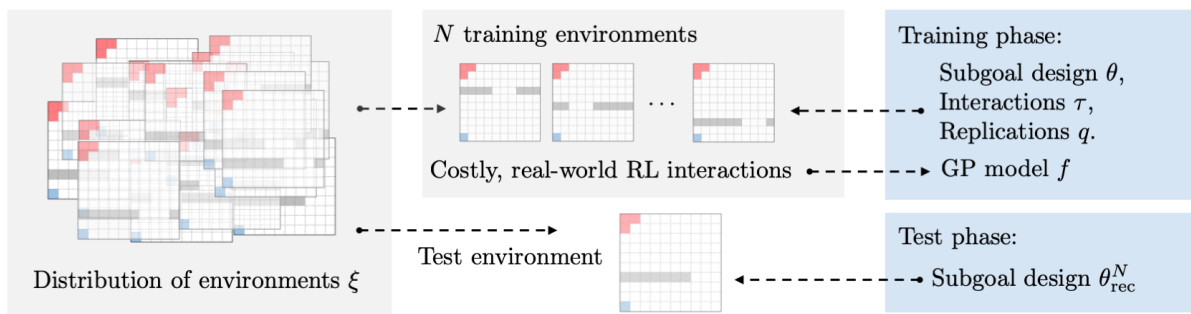
Figure 2: Outline of the BESD algorithm. During the training phase BESD optimizes an exploration strategy (represented as subgoals) on sampled training environments. It then utilizes the learned subgoal design as an exploration strategy in the test environment to train an effective policy within a limited number of interactions.
