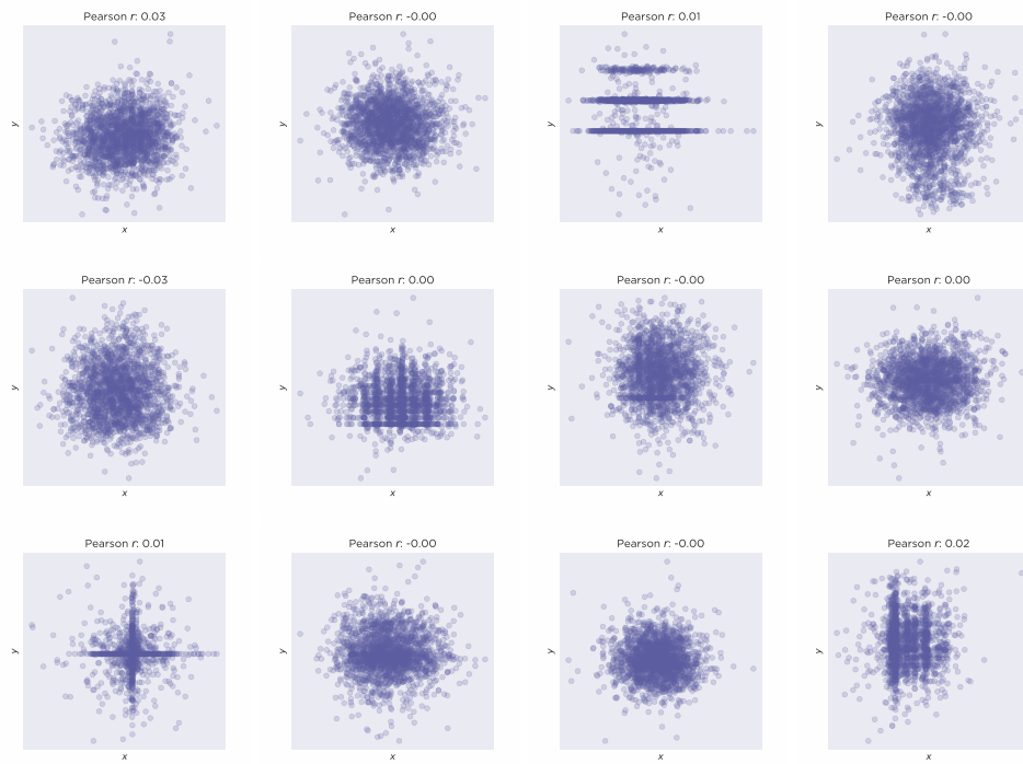
Figure A.2: The scatter plot and correlation between the signal pairs illustrated in Fig. A.1). The correlation (Pearson's r ) between is almost always approx. 0, indicating non-linear dependence.
