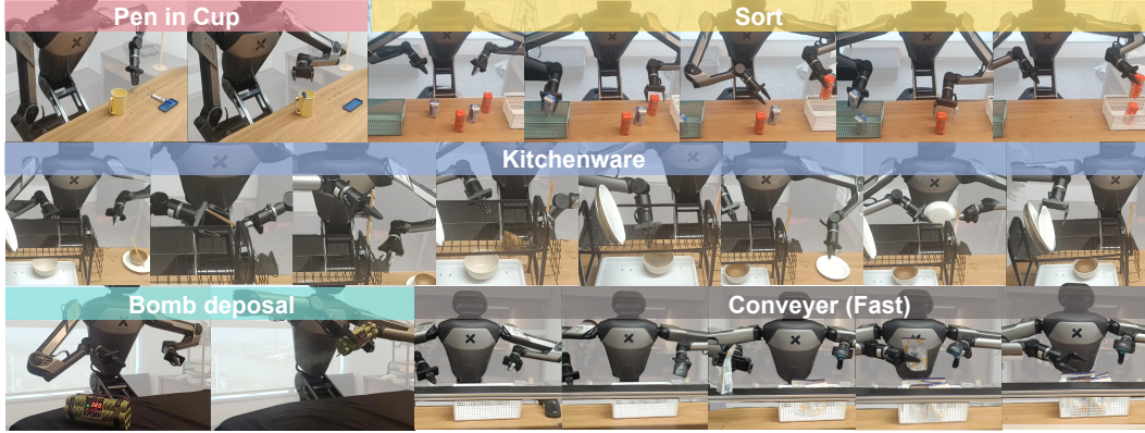
Figure 4: Real-world Setup. We consider five real-world challenging tasks. Sort , Kitchenware emphasize long-horizon manipulation that require multiple skills. Bomb Deposit requires precise manipulation. Conveyer and its variation Conveyer Fast is sensitive to manipulation speed.
