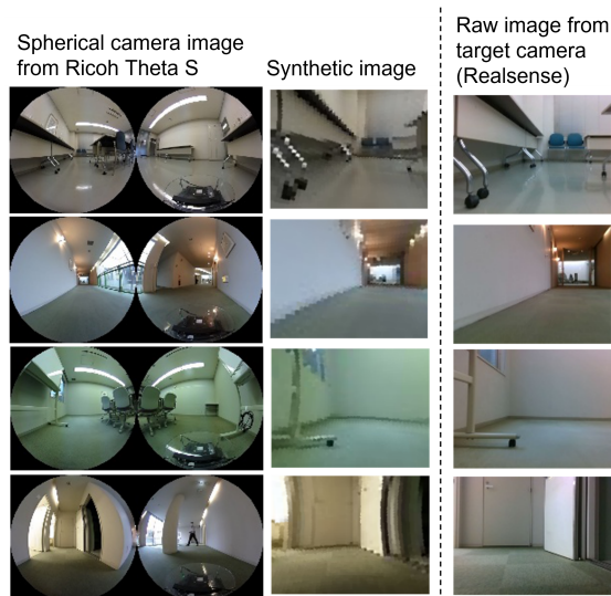
Fig. 7: Comparison of the synthetic images with the raw images of the target camera, Realsense. We mount the spherical camera and the Realsense at different positions on our robot platform. We generate synthetic images corresponding to the Realsense from the spherical camera images.
