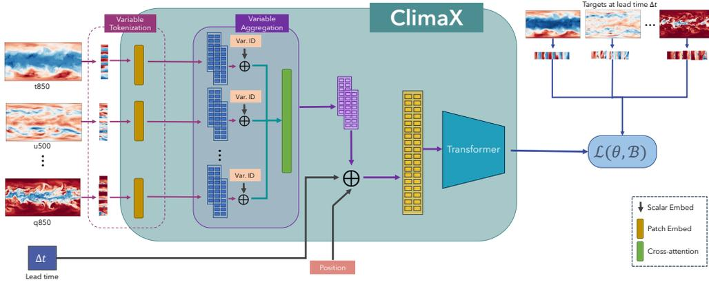
Figure 3. Pretraining phase of ClimaX. Variables are encoded using variable-separate tokenization, and subsequently aggregated using variable aggregation. Together with position embedding and lead time embedding those are fed to the ViT backbone.
