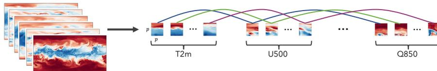
Figure 2. Variable tokenization tokenizes each variable independently, and variable aggregation reduces the sequence length by  $V$ .
