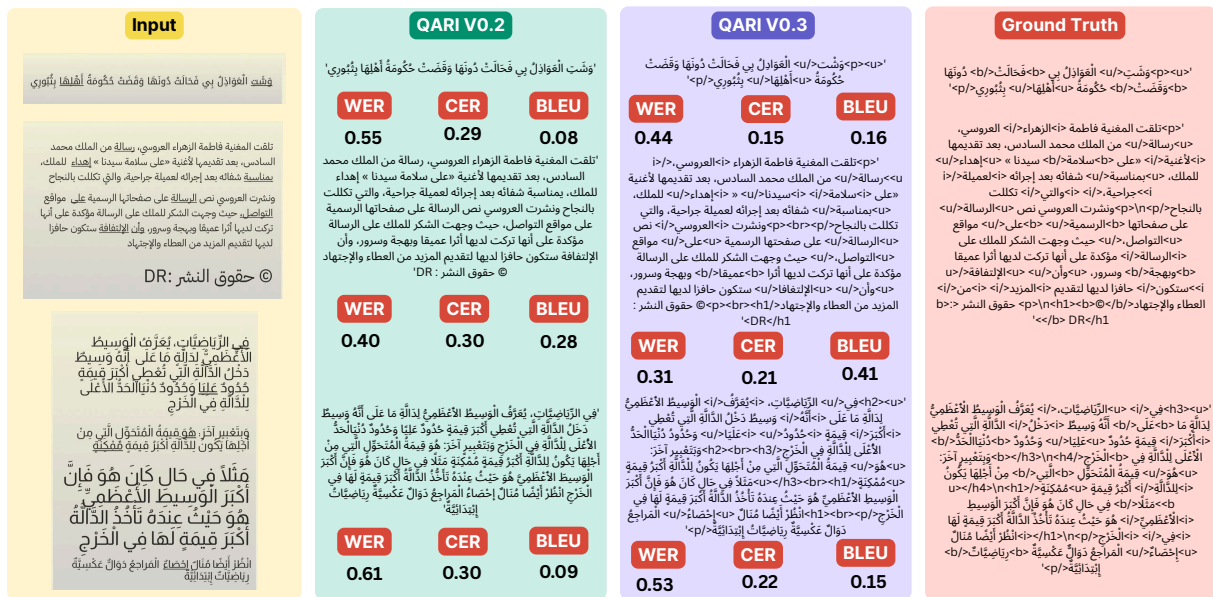
Figure 5: Qualitative comparison of QARI v0.2 and QARI v0.3 outputs against Input and Ground Truth for various Arabic text samples.
