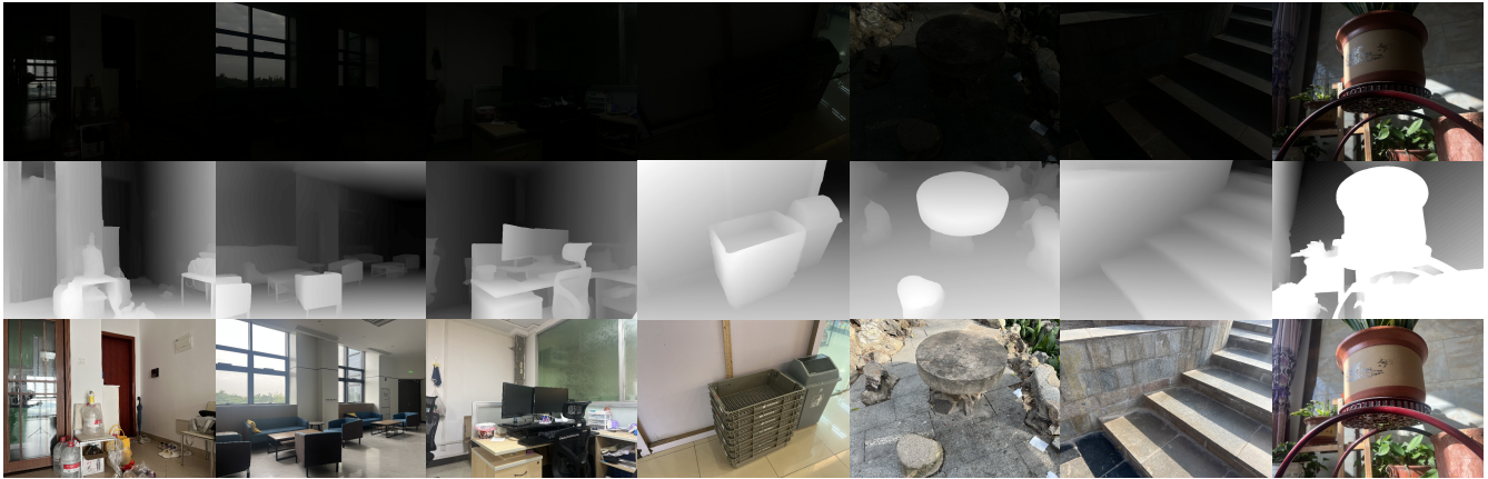
Figure 1: Some samples from LED dataset. The first row is the low-light RGB image, the second row is the depth map (the darker colors indicate a greater distance from the camera), and the third row is the normal-light image.
