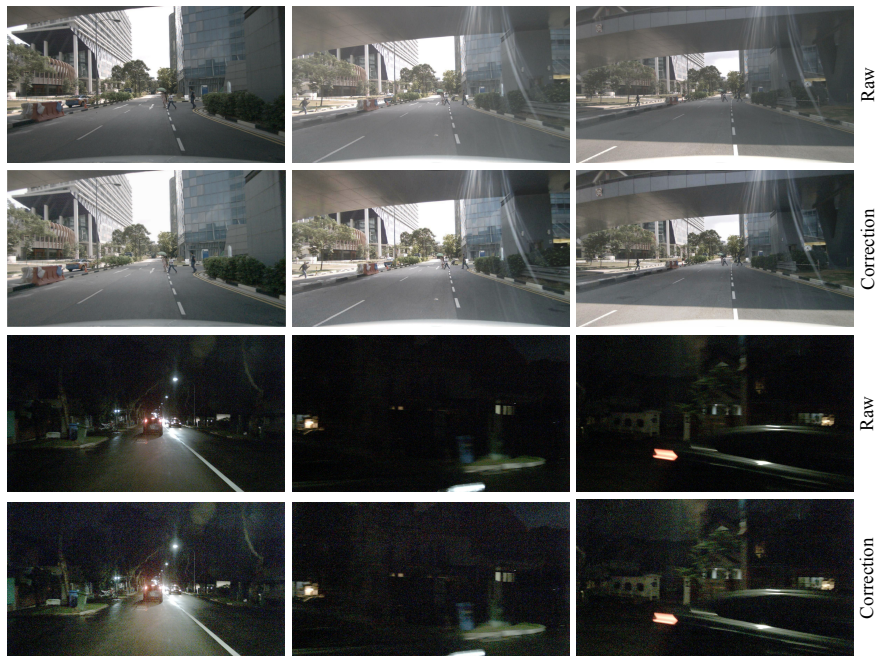
Figure 6: Qualitative display of images before and after Spatial-temporal Photometric Consistency Correction. The top two rows show the correction effect of three temporally adjacent images. The bottom two rows show the correction effect of spatially adjacent images in nighttime scenarios. Best viewed with zoom-in.
