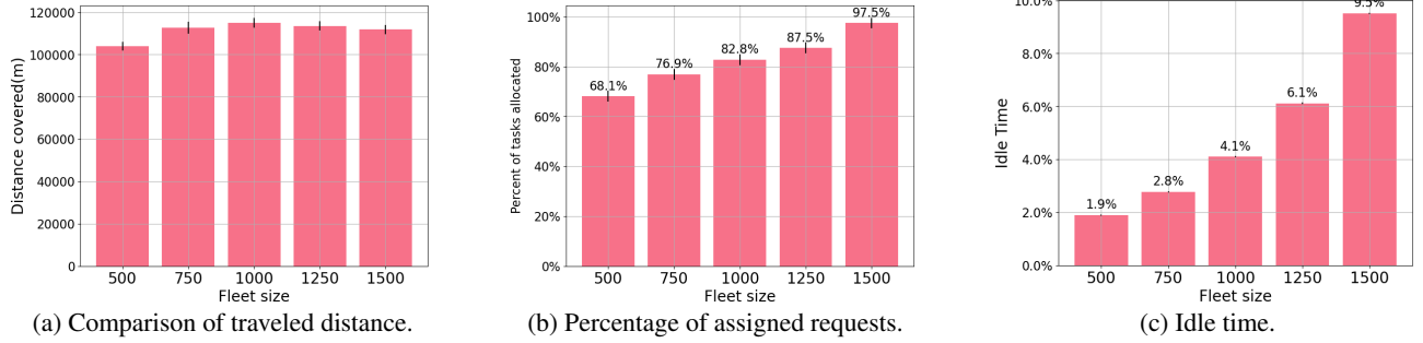
Figure 4: Comparison of the overall distance, number of assigned requests and idle time regarding the fleet size.
