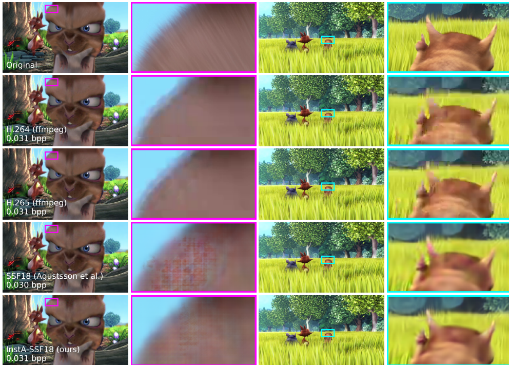
Figure 7: Original and compressed details in frames 7395 (left) and 7276 (right) of the Big Buck Bunny video (Xiph.org). From top to bottom, we compare the original, compressed frames with the H.264 and H.265 codecs in the ffmpeg (x264/x265) implementation, the SSF18 baseline, and our proposed InstA-SSF18 method. We use settings with comparable, low bitrates; the achieved bitrates (over the 10s sequence) are given in the left panels. All codecs lose textural details, but our InstA-SSF18 codec reduces the artifacts visible in the SSF18 reconstructions.
