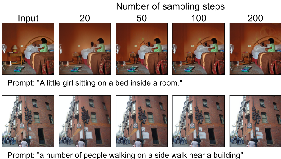
Figure 5: Reconstructed images when changing the number of sampling steps. The images become more similar to the input images as the number of sampling steps increases.
