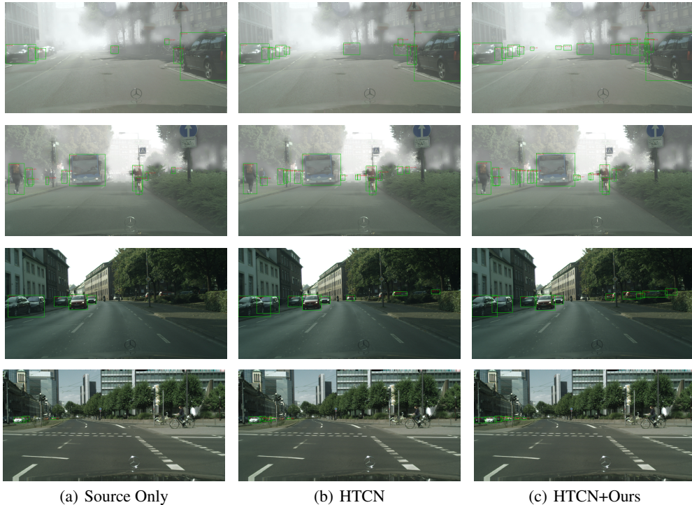
Figure 4: Qualitative detection results on the target domain. First and second rows: Normal→Foggy adaptation scenario. Third and fourth rows: Sim10K→Cityscapes adaptation scenario.
