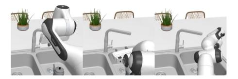
Figure 5: Snapshots over time from policy rollouts on the TurnOnSinkFaucet task in RoboCasa. Top: policy trained with Fourier features executes smooth and accurate rotations. Bottom: baseline policy without Fourier features struggles to complete the motion.
