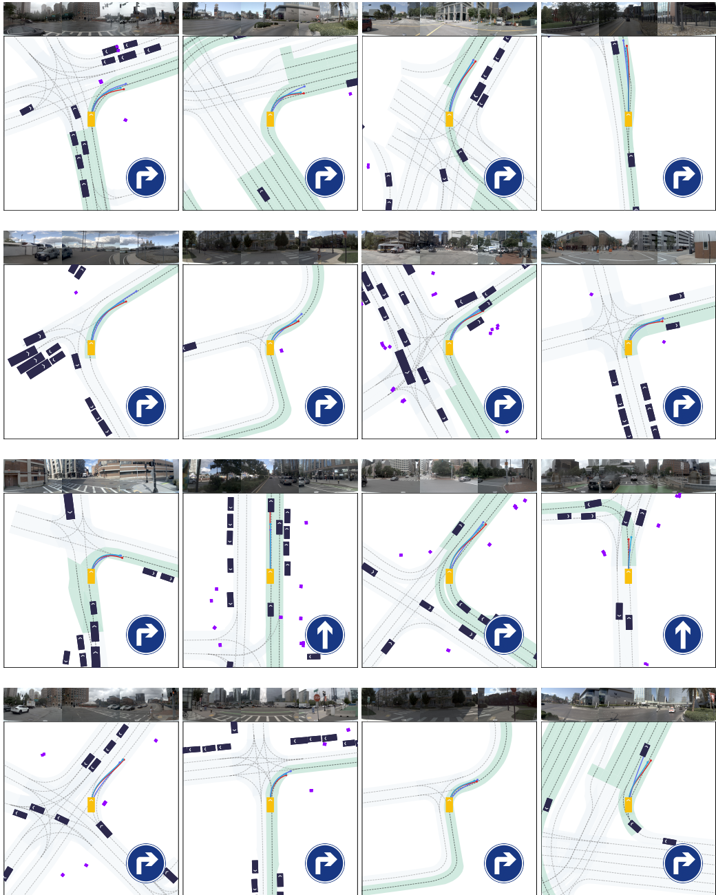
Figure 7: NAVSIM Results: DP-VLA w/ DIPOLE fine-tuned model trajectory; ground truth ego trajectory; DP-VLA imitation pre-trained model trajectory.
