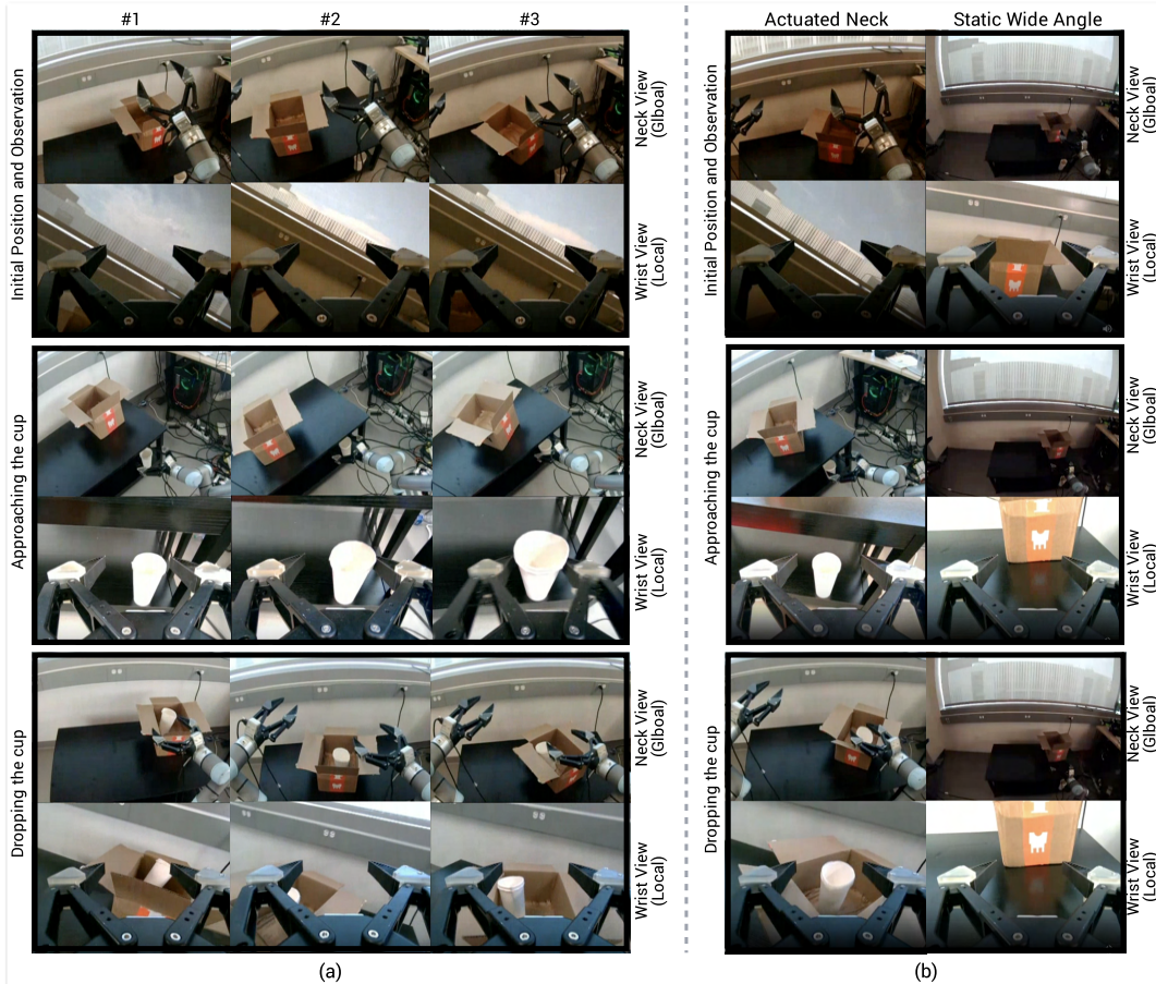
Figure 6: (a) Visualization of the autonomous execution of the task CFB across three different instances (columns #1, #2, #3). The actuated neck policy successfully generalizes to the three different instances of the task, despite the varying positions of the cup and the box highlighting its robustness. (b) Compares the autonomous execution of the task CFB with the actuated neck policy and the static wide angle lens policy. In the left column, the policy with the actuated neck successfully completes the task, dynamically adjusting the neck to guide the robot’s movements and place the cup inside the box. In the contrast, the robot with the wide angle policy fails to accomplish the task with the gripper getting stuck during the approach phase.
