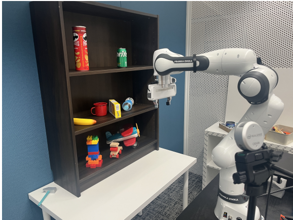
Figure 10: Hardware setup of our real world experiment. The Franka Emika Research 3 is placed in front of the scene and we use Realsense L515 pointing towards the scene to capture RGB-D information.
