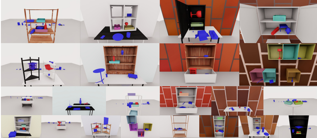
Figure 1: Examples of the fetching task in our benchmark. The red object is the target object that needs to be retrieved from the cluster to the free space in each task. Our scenes and tasks are generated with procedural rules, which mimic daily environments like shelves, cabinets, drawers, baskets, etc. The images are rendered with Isaac-Sim [8].
