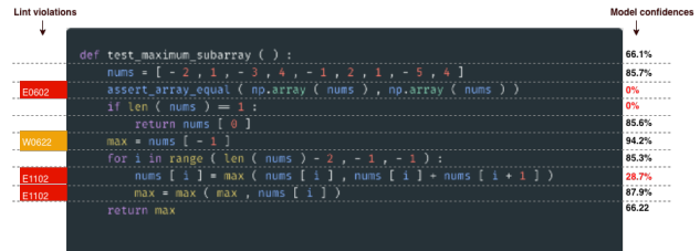
Figure 2. A code snippet translated from Java to Python3 with the corresponding Pylint errors and model confidences for each line. The max variable is used by the TransCoder output both as a variable and as the maximum operator. As we frequently found, little correlation is visible between model confidences (right) and lint violations (left). See Appendix A.3 for the Java source code, and Figure 5 in the Appendix for an enlarged image.
