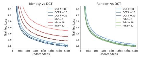
Figure 5: Training loss with different linear transformations. The left plot compares the DCT against the identity mapping, while the right plot compares the DCT with a random orthonormal projection matrices. Each curve corresponds to a different sparsity level  $k \in \{8, 16, 32\}$ .
