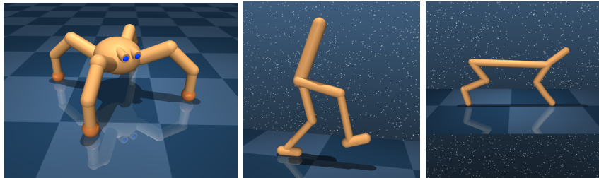
Figure 4: Domains used for evaluating zero-shot transfer performance: Quadruped, Walker, and Cheetah robots from URLB (Laskin et al., 2021). Transfer tasks involve performing movements such as walking, running, jumping, and flipping.
