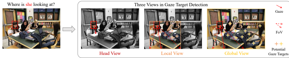
Fig. 2: Illustration of the head view, local view, global view in gaze target detection.
