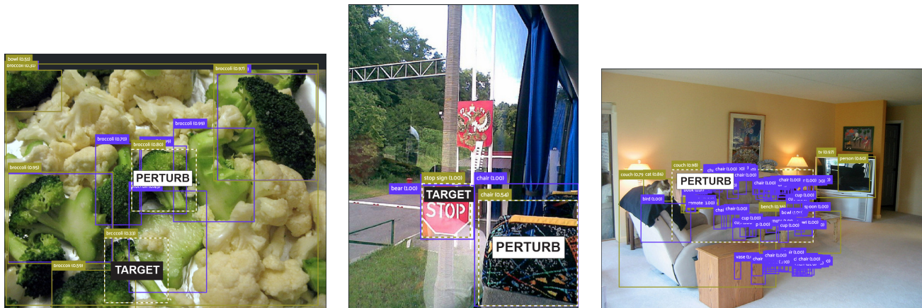
(a) A vanishing attack perturbs a broccoli and causes YOLOv3 to no longer detect the targeted broccoli (no purple detections are seen around the target).
