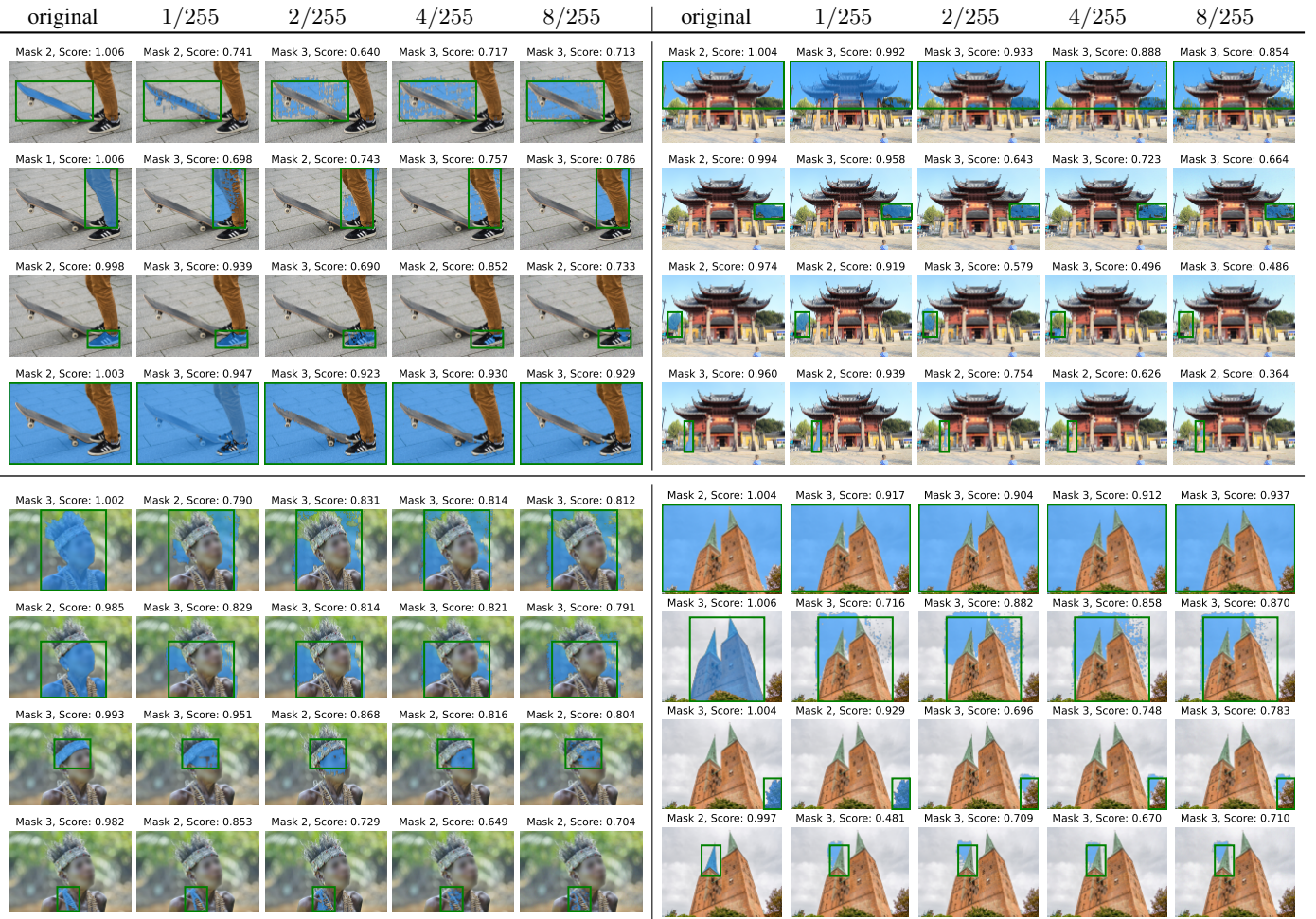
Fig. 5: Box prompts on SAM. We show the segmentation masks obtained with several box prompts and its quality score as in Fig. 3. We use either the original image or those perturbed with perturbations of \ell_\infty -norm \epsilon \in \{1/255, 2/255, 4/255, 8/255\} . Small perturbations effectively degrade the mask quality, especially for small and medium size objects.
