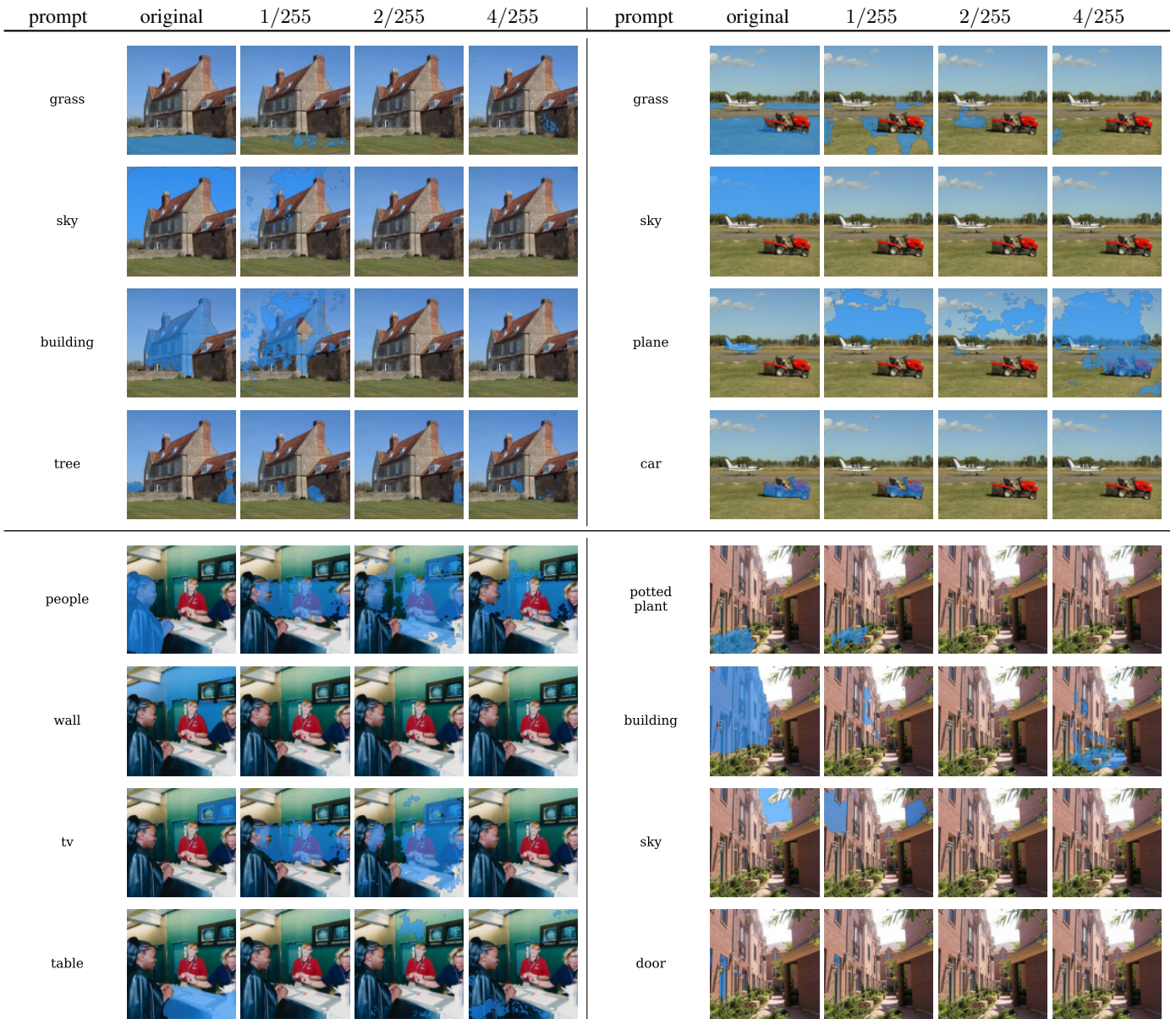
Fig. 9: Text prompts on SEEM (Focal-L). We show the predicted segmentation masks given several text prompts for both clean and adversarially perturbed (perturbation size \epsilon \in \{1/255, 2/255, 4/255\} ) images from ADE20K. While the original masks can precisely identify the objects for each class, small perturbations significantly alter the predicted masks.
