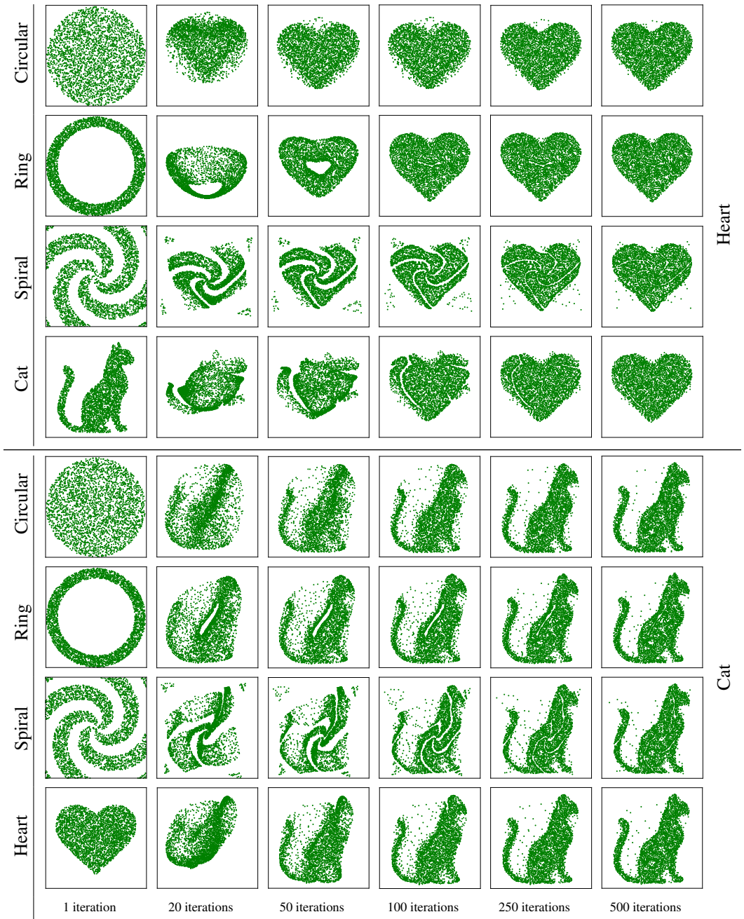
Figure 7: (Color online) Samples evolving with iterations for the discriminator-guided Langevin sampler, considering various shapes of the initial uniform distributions, given a target uniform distribution shaped like a Heart , or a Cat as indicated. For relatively simpler input shapes, such as the circular pattern, the sampler converges in about 100 iterations, while in the spiral case, the sampler converges in about 250 steps.
