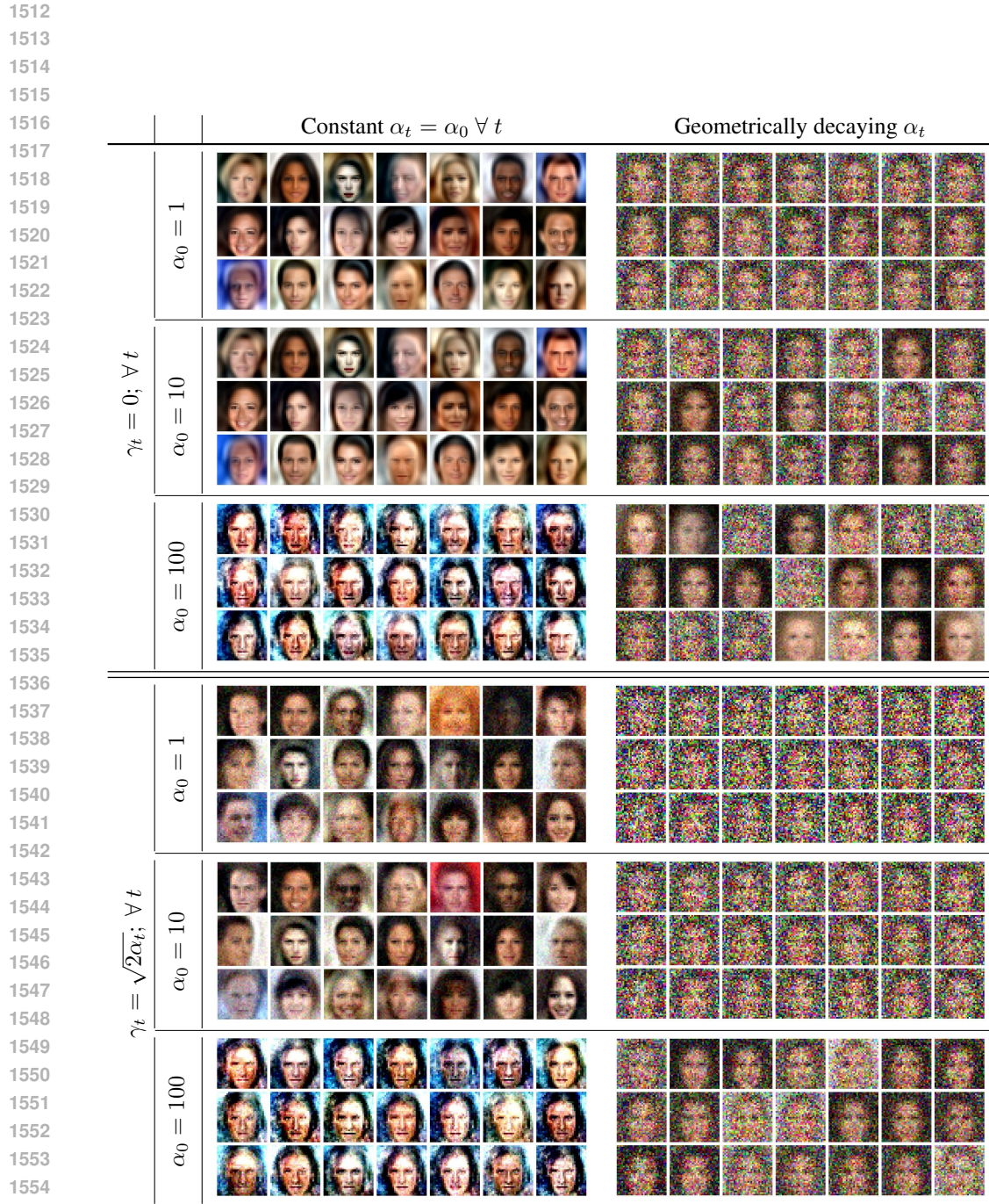
1556 Figure 10: (Color online) Images generated using the discriminator-guided Langevin sampler with 1557 CelebA as the target. The model fails to converge when \alpha_t decays geometrically, or when z_t \neq \mathbf{0} . 1558 Setting \alpha_0 \in [1, 10] , with z_t = \mathbf{0} results in the sampler generating realistic images. For these choices 1559 of \alpha_0 , when z_t \neq \mathbf{0} , the generated images are noisy.
