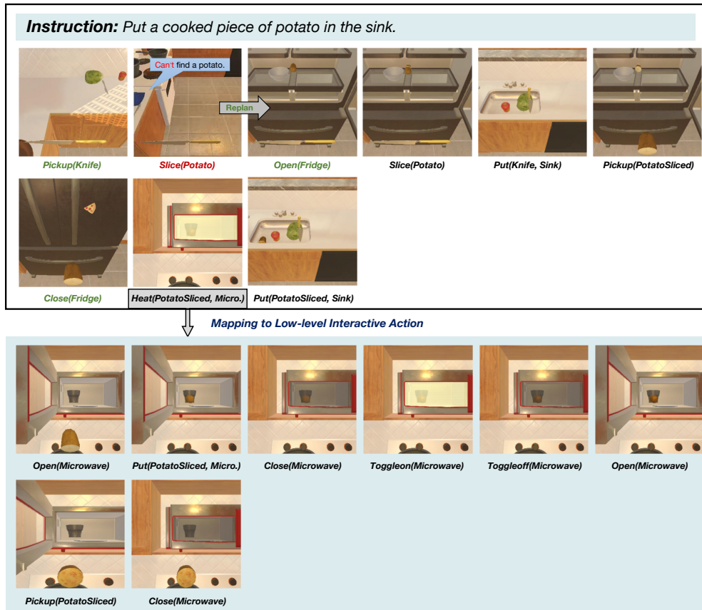
1239 Figure 8: An Example of GraphPlan on replanning: When the agent fails to locate a potato during 1240 environmental exploration while executing slice(potato), an error triggers the replanning process. 1241 The revised plan then attempts to open the refrigerator to search for one.
