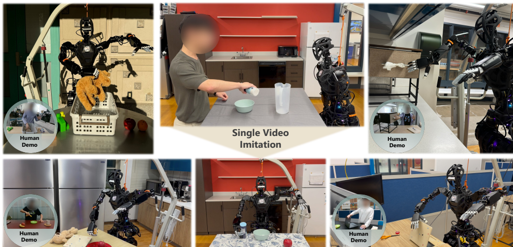
Figure 1: OKAMI enables a human user to teach the humanoid robot how to perform a task by providing a single video demonstration.
